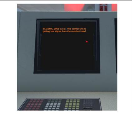
A close-up view of the MOP screen displaying a red alarm message: "ELCSMK_0001-La S: The control unit is getting low signal from the receiver head".                                             |
